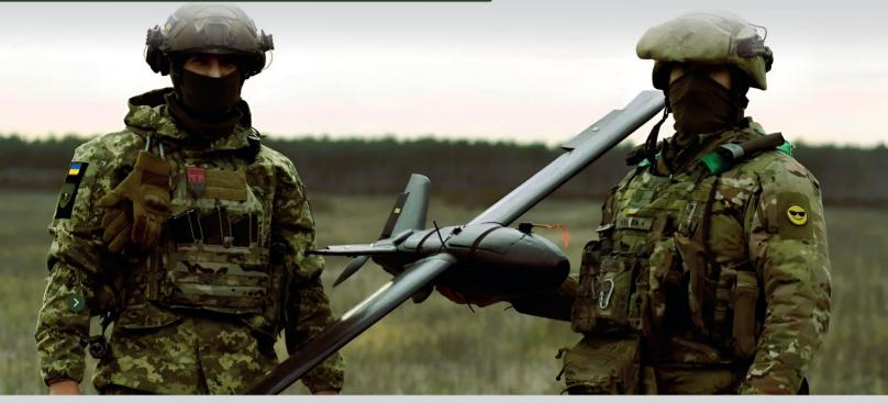
The UAV complex "Chaklun" is a multifunctional mobile system designed for conducting aerial visual reconnaissance. Thanks to the unmanned aerial vehicles (UAVs) included in the complex, it can carry out reconnaissance, patrol, correction, and search operations. Due to their small size and the radio-transparent material of the body, the aircraft are almost invisible on radars, allowing them to penetrate deep into enemy territory undetected.
