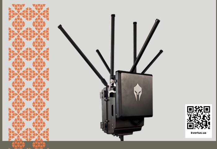
KVERTUS AD KRAKEN-E is a powerful portable dome-shaped and directional protection system against Mavic and low-cost Autel drone models, as well as against FPV drones using standard control frequencies.
